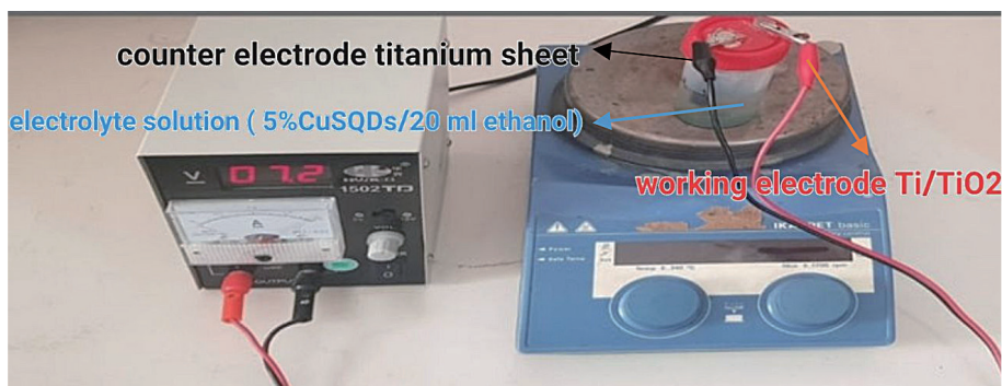
Fig. 2 The DC power supply 1502TD for Electrodeposition of CuS QD on the working electrode Ti/TiO 2 nanosheet surface.
